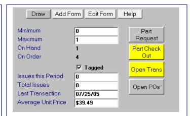
In the Parts Edit screen in the upper right corner, the Part Check Out button was added in version 4.36. This allows you to check out a part right from the parts screen. The only thing you need to add is the Equipment where the part was used.
